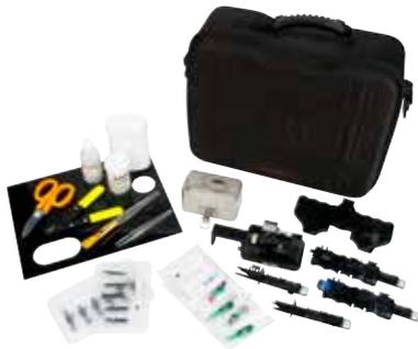
The 3M™ Fiber Optic Angle Cleave Kit 2565 includes the 3M™ Fiber Optic Angle Cleaver 2535 and all tools necessary for 3M™ No Polish Connector 8800-APC/AS
