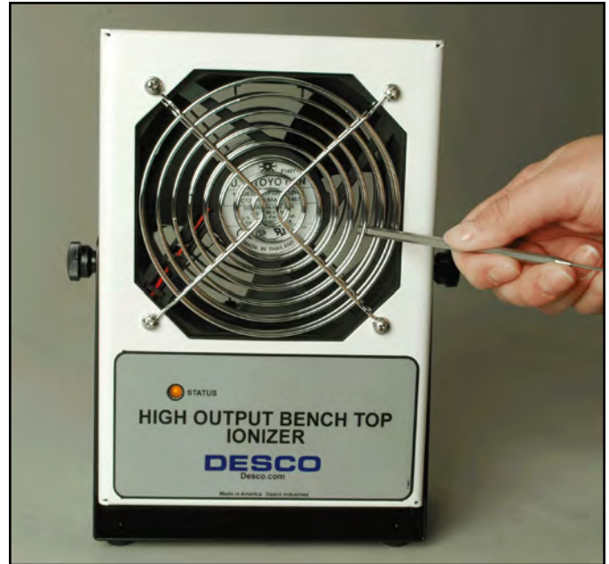
Figure 7. Shorting the ionizer's fan grills with a metal probe to test the alarm
