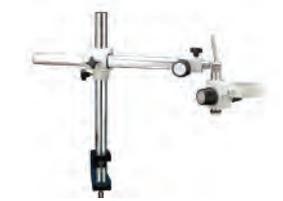
**23731**, this model has all the same features as the 23730 Boom Stand except it comes with a heavy-duty clamp mount instead of a base. Clamp opens up to 4" wide to attach to workstations or bench edges.
