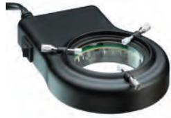
**18744**, LED Ring Light maximizes light output and distribution while preventing harmful glare and reflections. Its modular construction and brilliant 40 LED display makes this ring light ideal for the inspection of surface cracks and defects. Pure-white LED lights have a 50,000 hour lumen maintenance (lamp life). 6000°K color temperature is perfect for lead free inspection and a removable/replaceable diffuser allows for easy cleaning.
