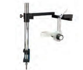
**23732**, the Articulating Arm Stand has a heavy-duty mount that opens up to 4" wide to mount to workstations or bench edges. The horizontal reach is over 36" when fully extended (measured from vertical post to the middle of microscope body) and its maximum clearance is 14" above the worksurface. This is one stand that truly frees valuable bench space and still gets the microscope out where it's needed for assembly and rework.
