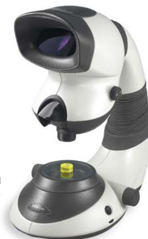
High stability bench stand, with integral focus and dimmable substage illumination.
