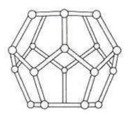
Plastazote® is a closed cell, cross-linked polyethylene foam manufactured using Zotefoams unique production process.
