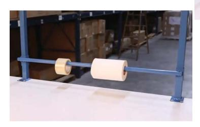
Fit the holes in the ends of the roll bar onto the posts on the brackets.
