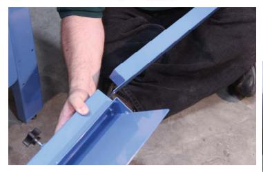
Select the desired adjustment holes on the base of the leg pairs.
