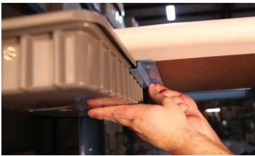
Replace the inside bin drawer rail, and retighten the 3 wood screws.
