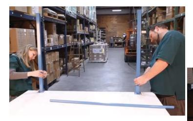
Loosen the thumb screw on each bracket and slide them over the end of each upright.
