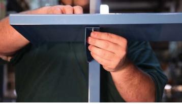
Align the shelf with the 4 holes in the shelf brackets, insert the bolts, and attach the washers and nuts.
