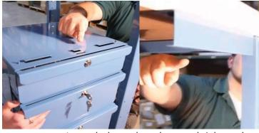
Insert bolts and washers and tighten the drawer stack to the back mounting bracket on the underside of the bench top.
