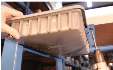
Remove the 3 wood screws loosely holding the inside bin drawer rail.
