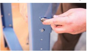
Do the same for both sides of each leg pair, making sure to keep the leg height consistent.
