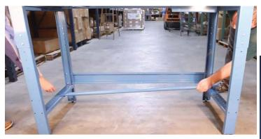
Insert bolt and attach thumb screw
