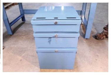
Hold in place and slide the top most drawer forward exposing 2 holes on the back mounting bracket.
