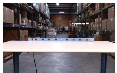
The power strip attaches to the back of the bench top using 4 small wood screws.
