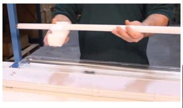
Remove each bulb, discard the foam packing, replace the bulbs, and reassemble the housing.
