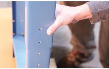
Insert the bolts with the lock washers on the inside of the leg and tighten the nuts until the lock washers are flat. (4 total bolts per leg pair, 2 bolts each side)
