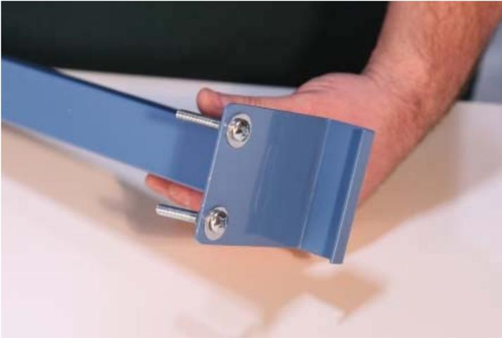
Fit the bracket on the end of the upright over the back edge of the bench top and align with the predrilled holes.
