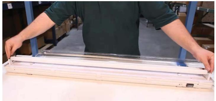
Remove each bulb, discard the foam packing, replace the bulbs, and reassemble the housing.
