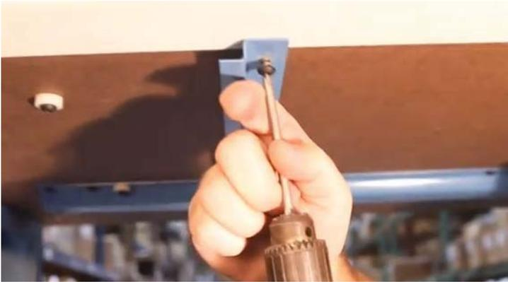
Remove the 3 wood screws loosely holding the inside bin drawer rail.
