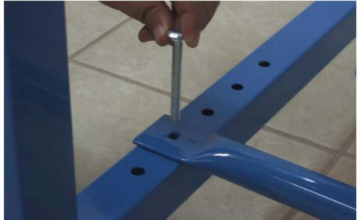
The square flange on the bolt should seat in the square hole on the footrest.
