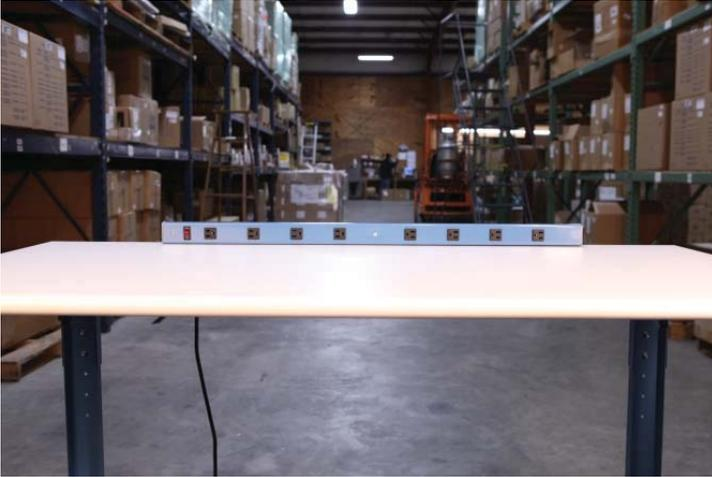
The power strip attaches to the back of the bench top using 4 small wood screws.
