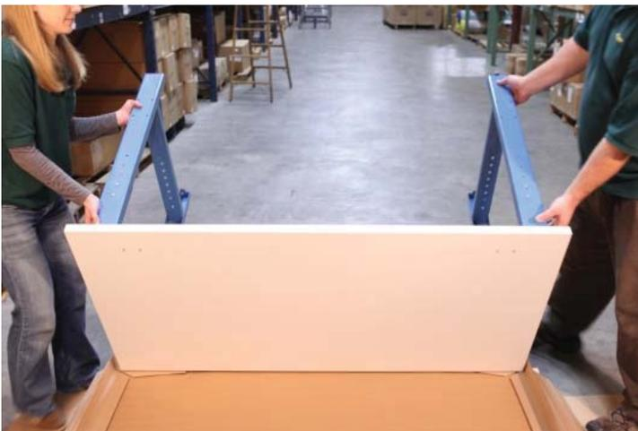
Open and unfold the top of the bench top packaging. You should see the underside of your bench top.
