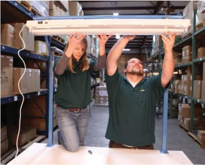
With the help of a second person, carefully lift the light assembly and hang the bracket onto the light frame.
