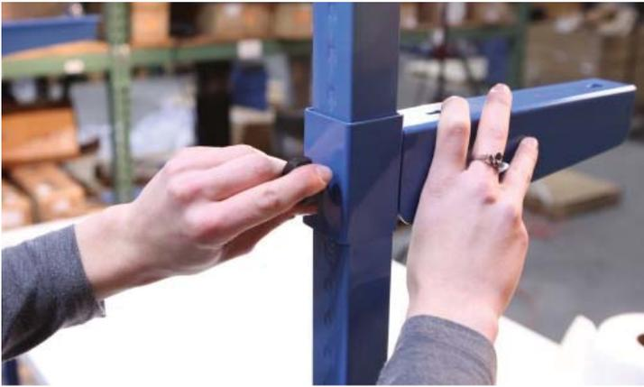
Loosen the thumb screws on the back of each shelf bracket and slide them over the end of each upright. Align to the desired height notch and tighten.
