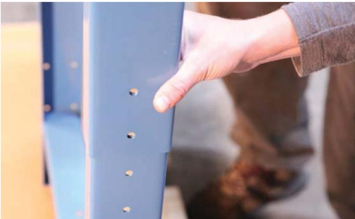
Insert the bolts with the lock washers on the inside of the leg and tighten the nuts until the lock washers are flat. (4 total bolts per leg pair, 2 bolts each side)
