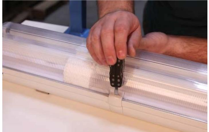
Loosen the thumb screws on the brackets, slip the light frame over the tops of the uprights, and tighten the thumb screws.
