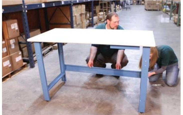
Each side attaches to the holes on the lower half of each leg using 4 bolts with lock washers.
