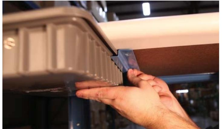
Replace the inside bin drawer rail, and retighten the 3 wood screws.
