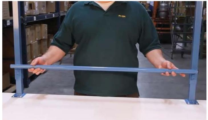
Fit the holes in the ends of the roll bar onto the posts on the brackets.
