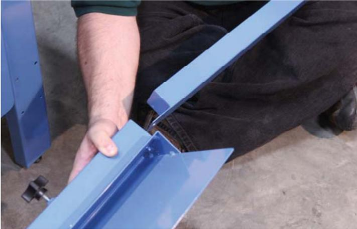
Select the desired adjustment holes on the base of the leg pairs.
