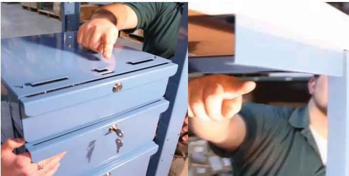
Hold in place and slide the top most drawer forward exposing 2 holes on the back mounting bracket.
