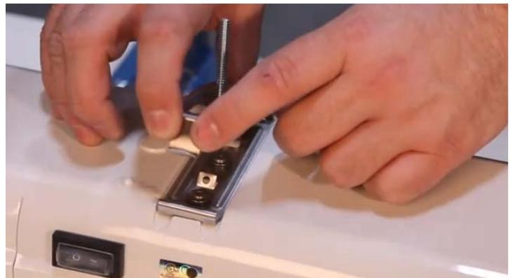
Attach the housing bolts through the holes in the light frame and tighten.
