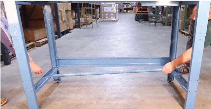
Insert bolt and attach thumb screw to the underside of the leg.
