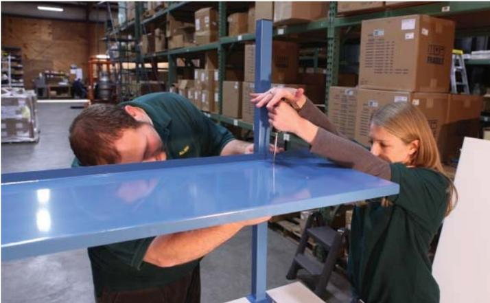
Align the shelf with the 4 holes in the shelf brackets, insert the bolts, and attach the washers and nuts.
