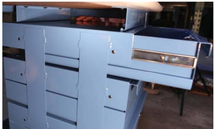
Insert bolts and washers and tighten the drawer stack to the back mounting bracket on the underside of the bench top.
