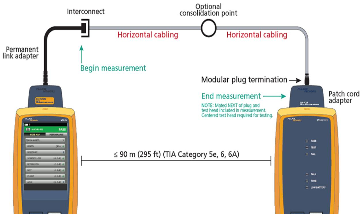
The patch cord adapters support Category 5e, 6, and 6A performance levels and work with all DSX CableAnalyzer™ models. The latest version of the Versiv/DSX firmware is required to use the MPTL testing limits.
