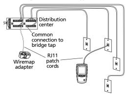
Note: For a correct length reading, connect the tester and wiremap adapter as shown. See the Users Manual for details.
