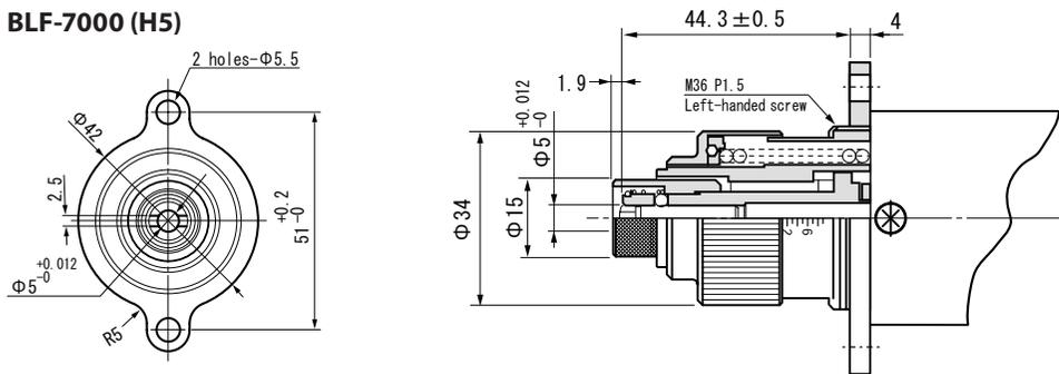
\* The flange can be removed by rotating it clockwise.
