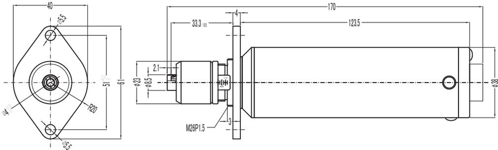
\* The flange can be removed by rotating it counterclockwise.
