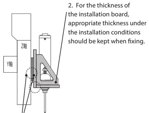
2. For the thickness of the installation board, appropriate thickness under the installation conditions should be kept when fixing.
