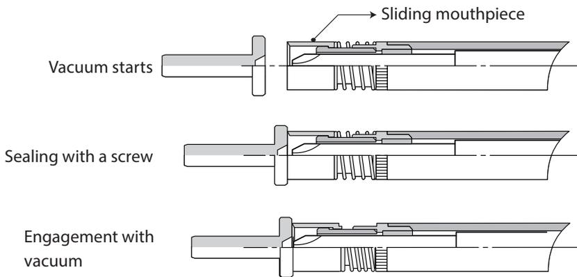
The sliding mouthpiece moves horizontally to hold the screw head and keeps it straight.
