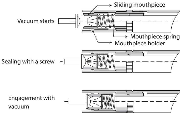
The sliding mouthpiece moves horizontally to hold the screw head and keeps it straight.
