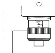
Torque adjustment nut can be turned and moved manually with this ring
