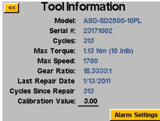
All the information shown on the screen above is stored on the internal memory of the SD250 screwdriver itself, and therefore travels with the tool when taken from one controller to another.
