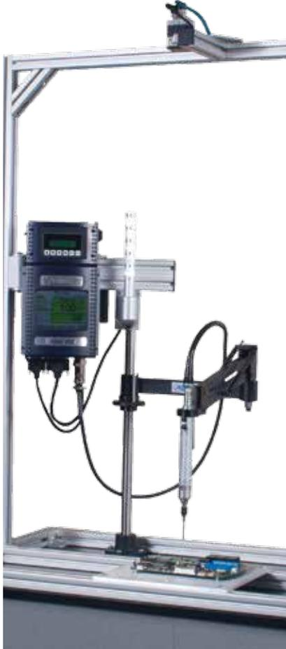
The sequence recognition system is the solution for applications such as those requiring uniform compression of all components within your product assembly. The ASG SRS ensures that the operator installs fasteners in a specific pre-programmed sequence.
