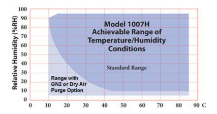
NOTE: Ability to reach RH extremes may be limited by the humidity sensor accuracy. Low Dew Point conditions can only be achieved when starting with a clean, dry chamber.
