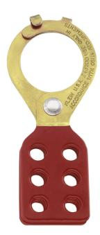
The Klein Tools Lockout with Interlocking Tabs is designed to lock out power sources, such as disconnects, switches and panel boxes. The lockout has zinc-plated double interlocking hasps of tempered steel with interlocking tabs for extra security. Tabs feature 6-hole locking bodies coated with red vinyl plastic.
